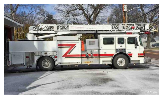
2003 American LaFrance Eagle, Ladder 75', Detroit turbo diesel, Allison automatic, air brakes, 2,000 gpm Waterous, 475 gal tank, FoamPro system, Pre-piped aluminum waterway w/ remote-controlled nozzle, (2) outriggers, generator, headset system, telescoping scene lights, Whelen warning lights, sirens. 29,840 miles. Asking \$149,000
