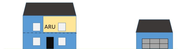
Example 3. Additional Residential Unit in Second Level
