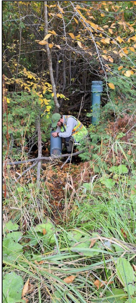
Quantitative sample #1 being collected using a modified T-sampler.
