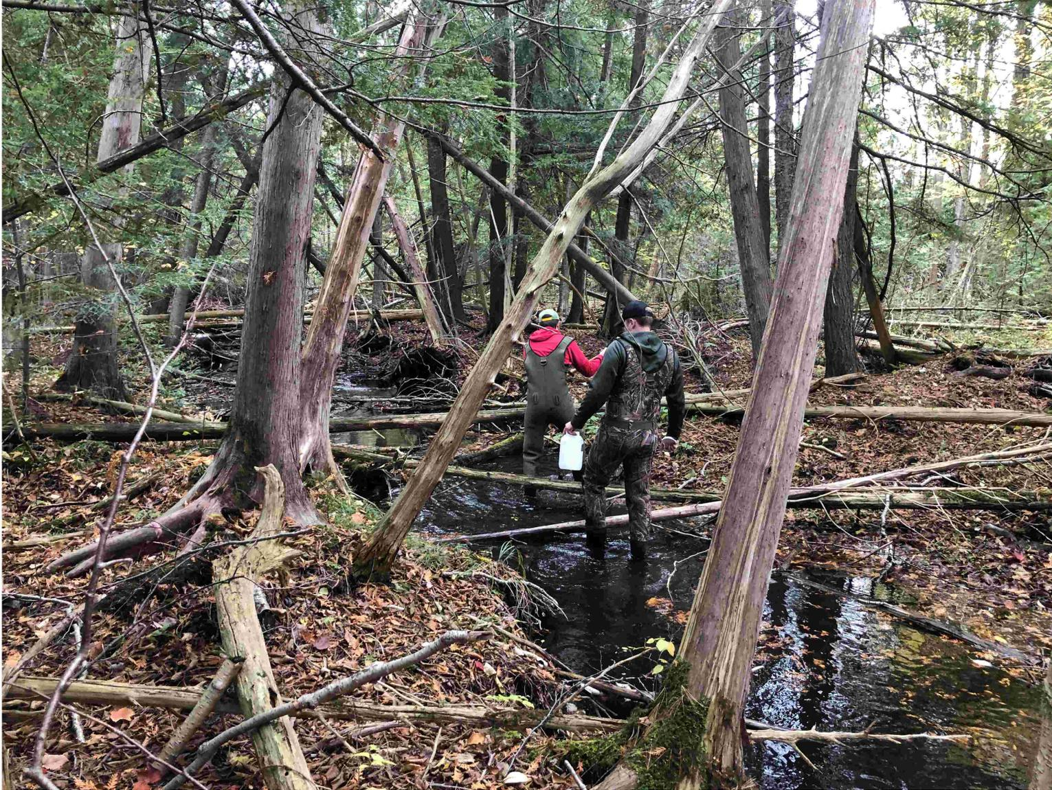
Oct 17, 2023 – Qualitative Sample collection using 60µm D-Net
