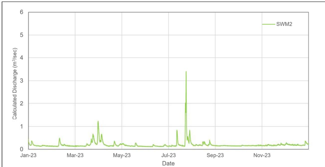
**Figure 2-4: 2023 Mill Creek Hourly Discharge at Surface Water Monitoring Station SWM2**
