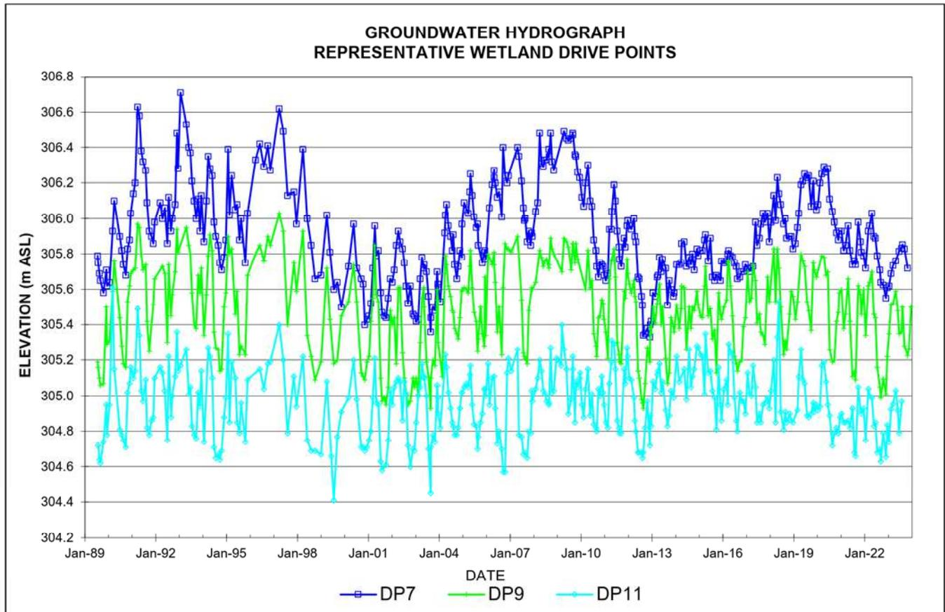
Figure 3-6: Groundwater Hydrograph of Three Representative Drive Points in the Wetland
