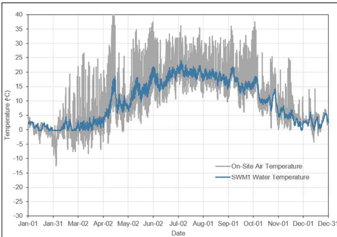
**Figure 3-17: 2023 Air and Water Temperature at SWM1**
