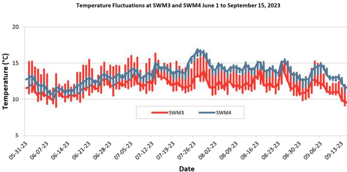
**Figure 4-3: Diurnal Temperature Fluctuations from June 1 to September 15, 2023 at SWM3 and SWM4**
