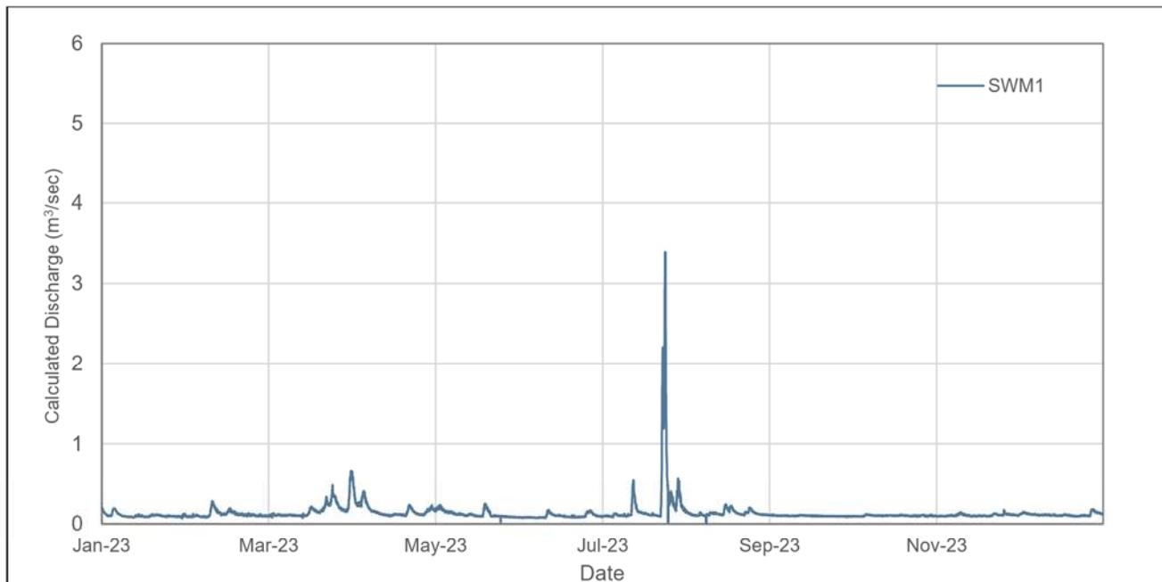
**Figure 2-3: 2023 Mill Creek Hourly Discharge at Surface Water Monitoring Station SWM1**
