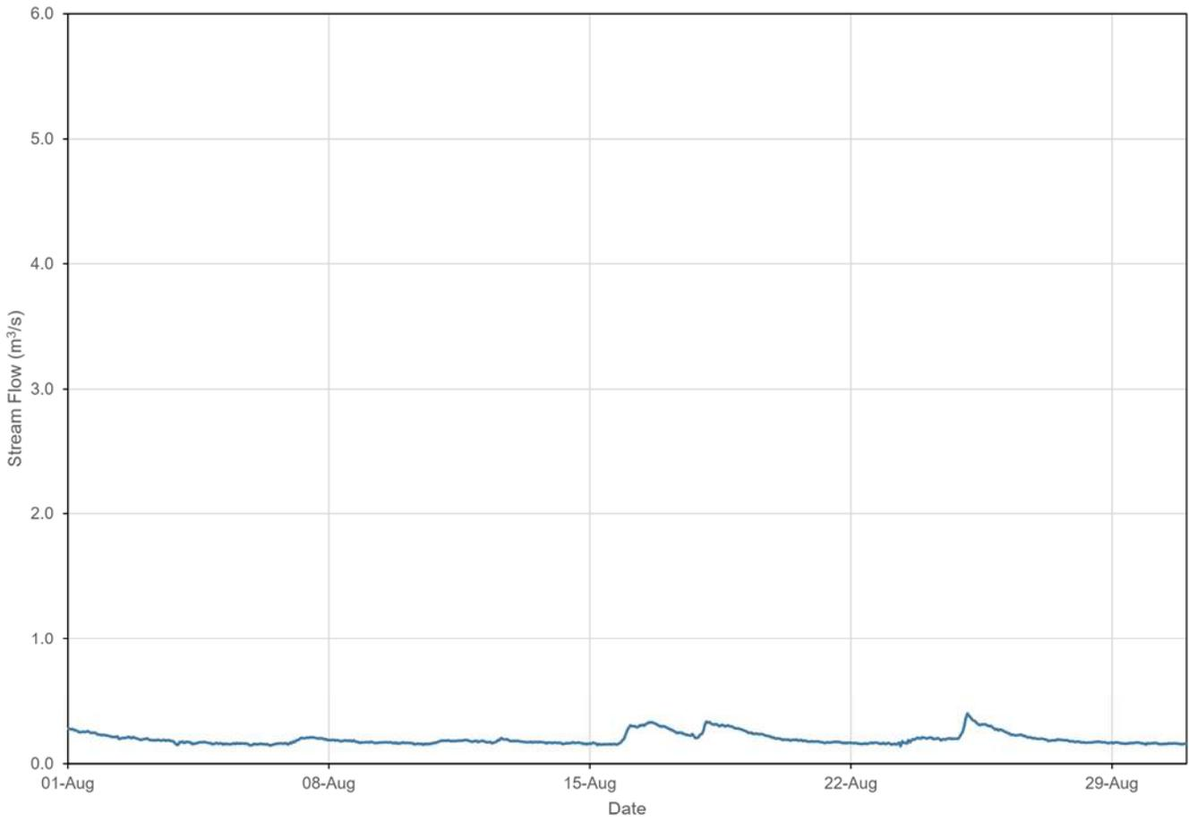
Figure C-21: 2023 Calculated Stream Flow at SWM2
