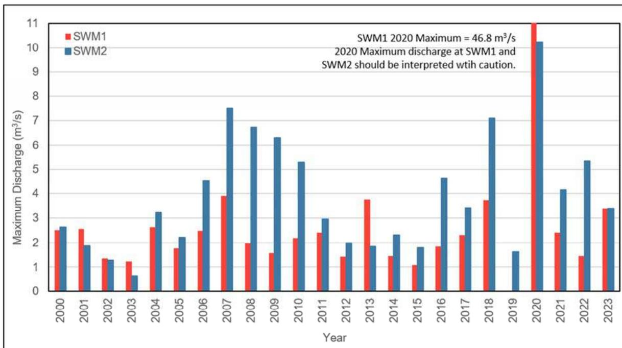
**Figure 2-8: Instantaneous Maximum Stream Discharge at SWM1 and SWM2, 2000 through 2023**
