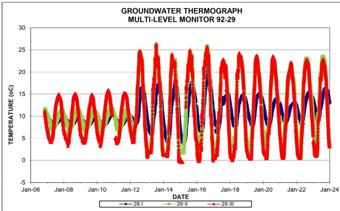
**Figure 3-2: Groundwater Thermograph of Multi-level Monitor 92-29**
