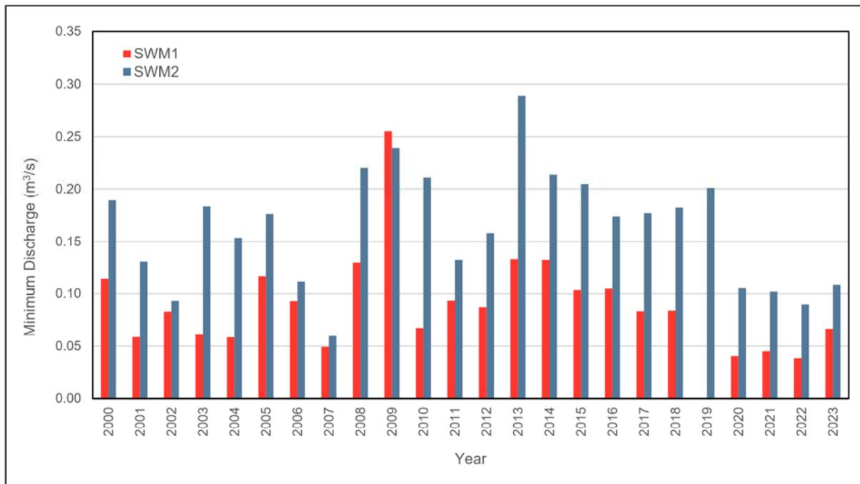
**Figure 3-11: SWM1 and SWM2 Instantaneous Minimum Stream Discharge (2000-2023)**
