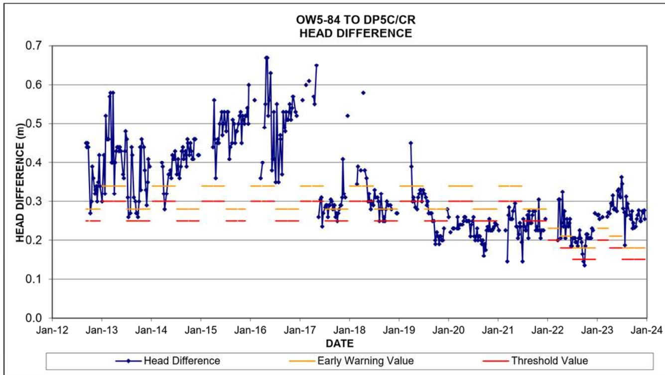
**Figure 3-15: Hydraulic Head Difference for Monitoring Pair OW5-84/DP5C/CR; September 2012 to December 2023**
