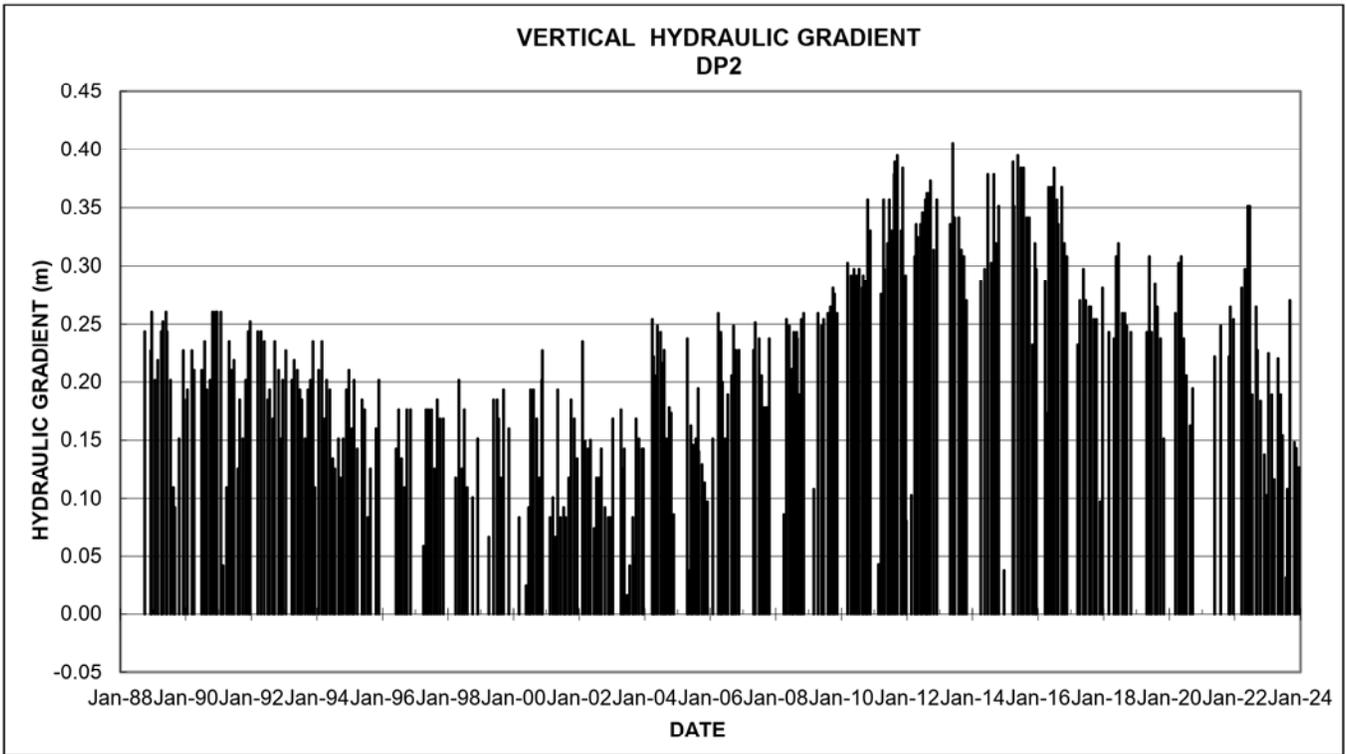
Figure 3-7: Hydraulic Gradient at Stream Drive Point Station DP2
