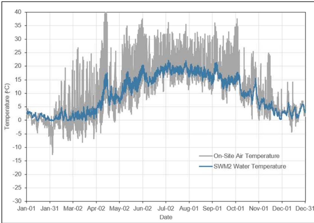
Figure 3-18: 2023 Air and Water Temperature at SWM2
