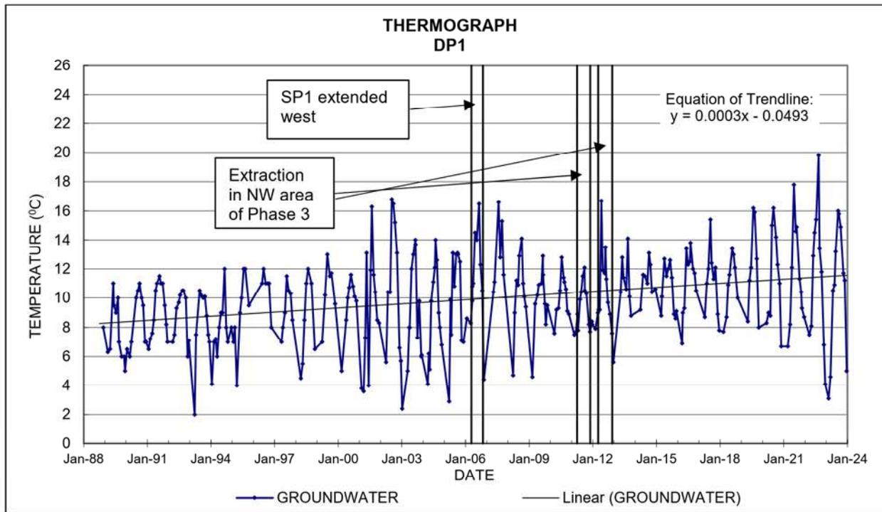
Figure 3-3: Groundwater Thermograph of Drive Point DP1
