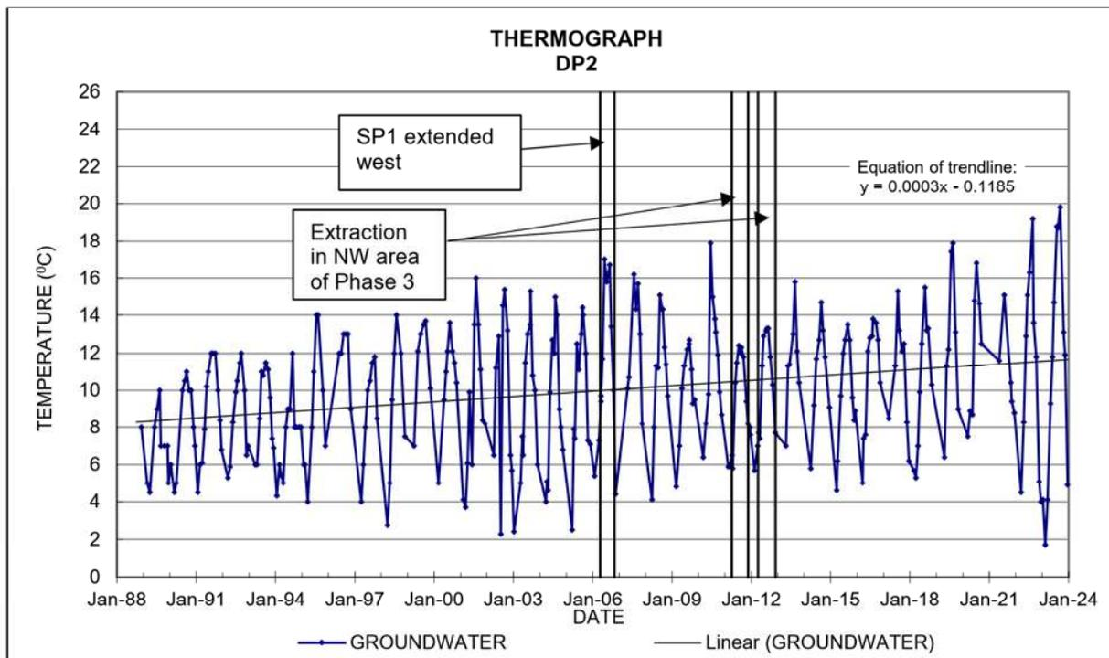
Figure 3-4: Groundwater Thermograph of Drive Point DP2
