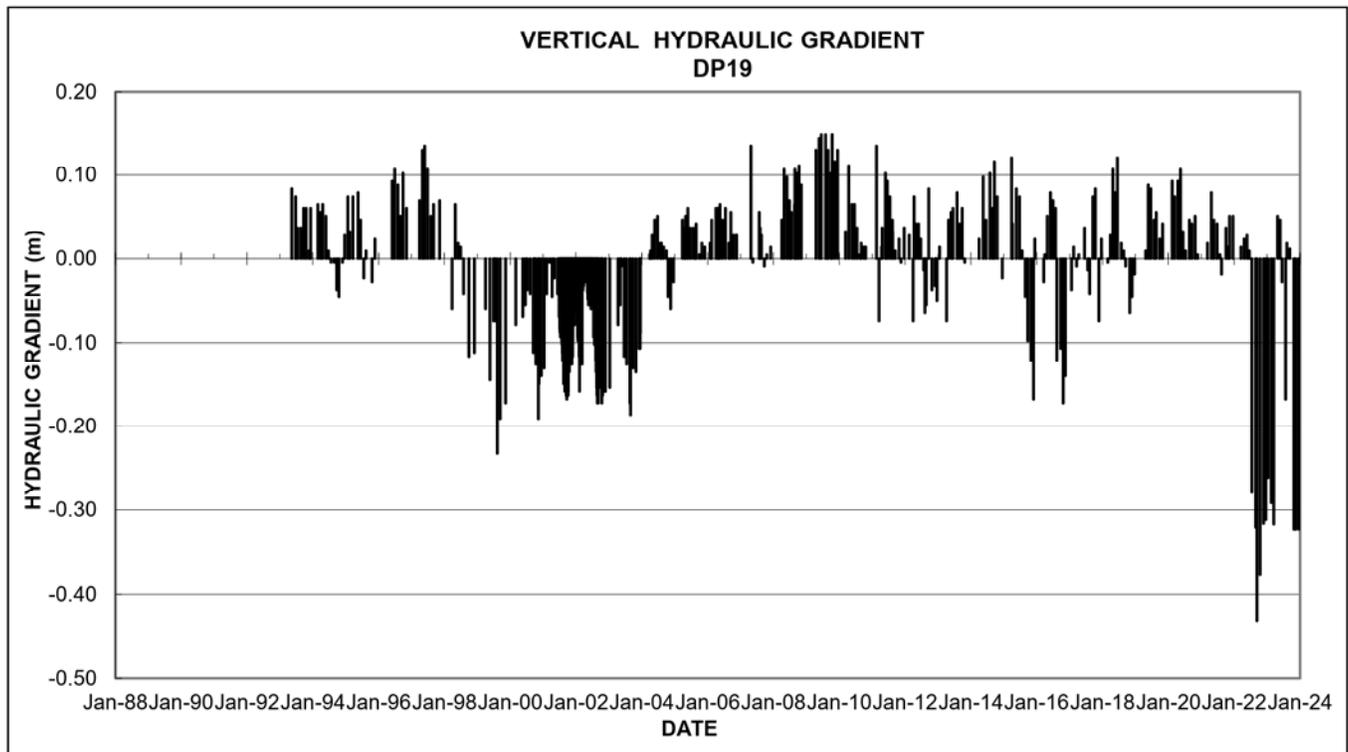
Figure 3-10: Hydraulic Gradient at Stream Drive Point Station DP19
