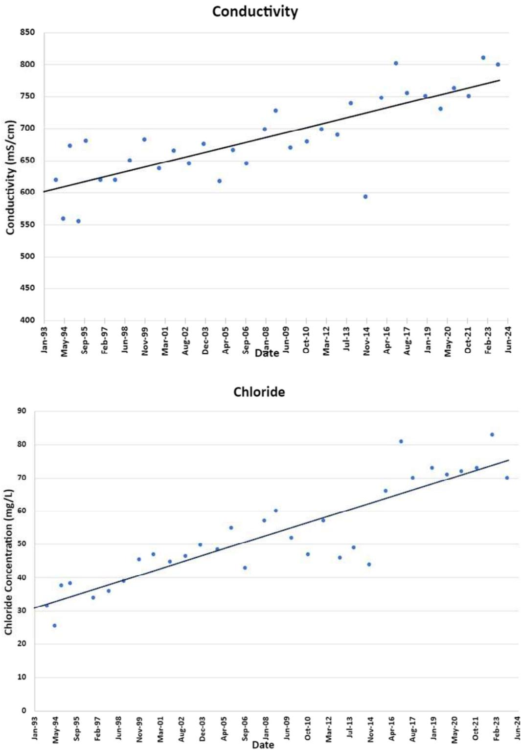
Figure 2: Historical Conductivity and Chloride Values in Mill Creek at SWM2 (1993-2023)
