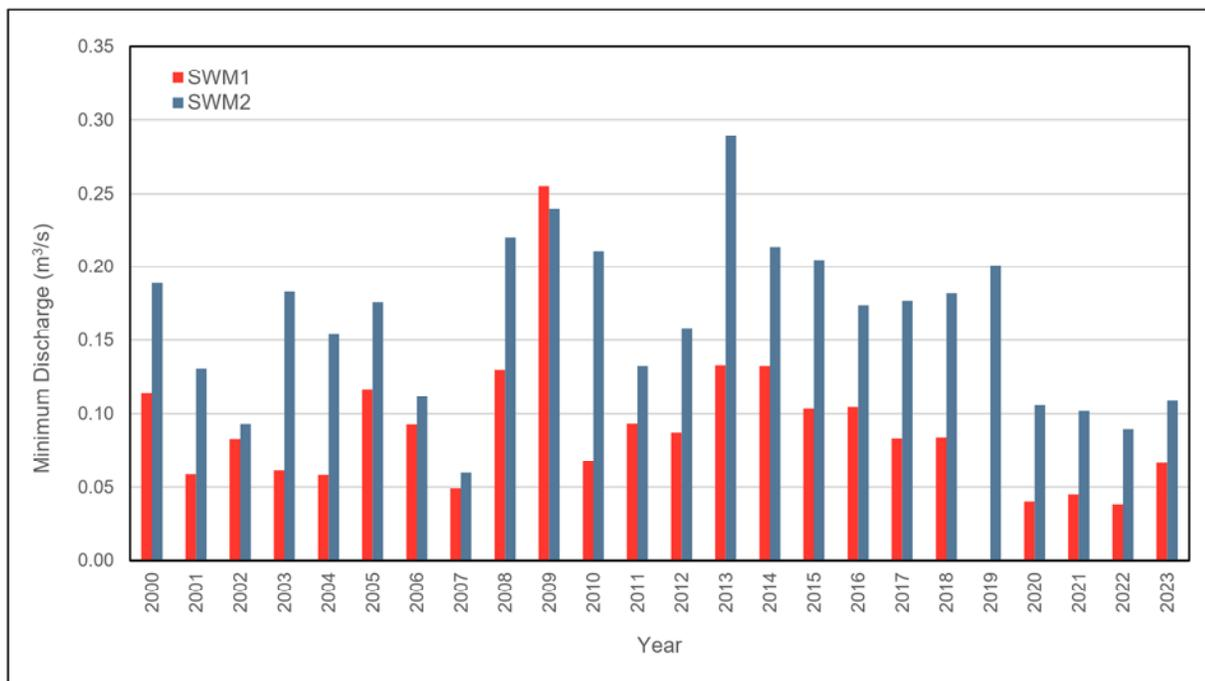
**Figure 2-7: Instantaneous Minimum Stream Discharges at SWM1 and SWM2, 2000 through 2023**
