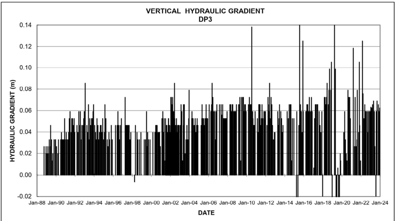
Figure 3-8: Hydraulic Gradient at Stream Drive Point Station DP3
