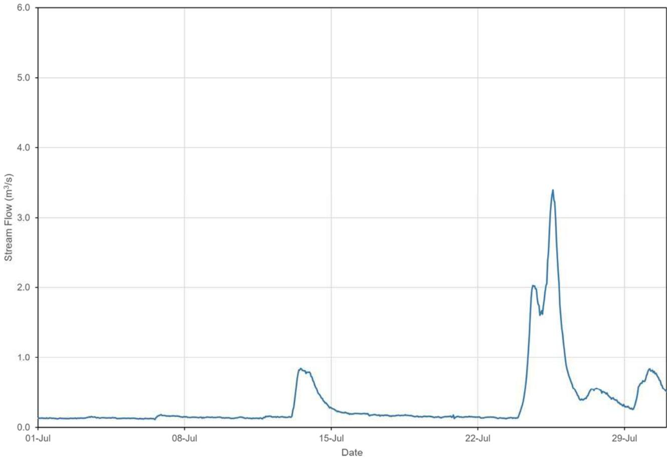
Figure C-20: 2023 Calculated Stream Flow at SWM2
