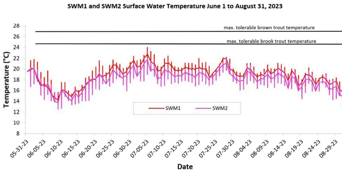
**Figure 3: Thermographs from SWM1 and SWM2, for June 1 to August 31, 2023**
