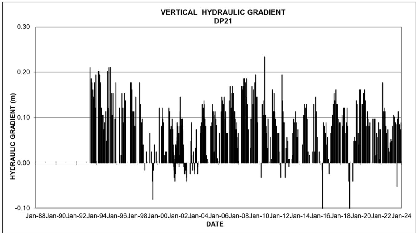
**Figure 3-11: Hydraulic Gradient at Stream Drive Point Station DP21**
