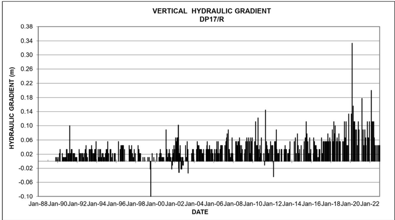
Figure 3-9: Hydraulic Gradient at Stream Drive Point Station DP17/R
