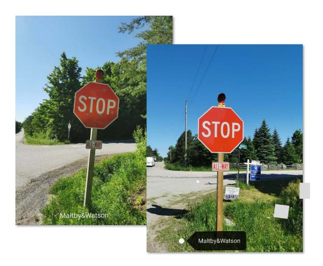
Figure 6.1: Stop Signs with Solar Powered Lights
