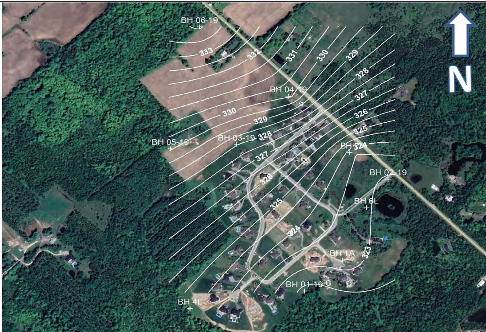
Drawing 3 - Groundwater Contours - September 2019 Audrey Meadows Subdivision - Puslinch
