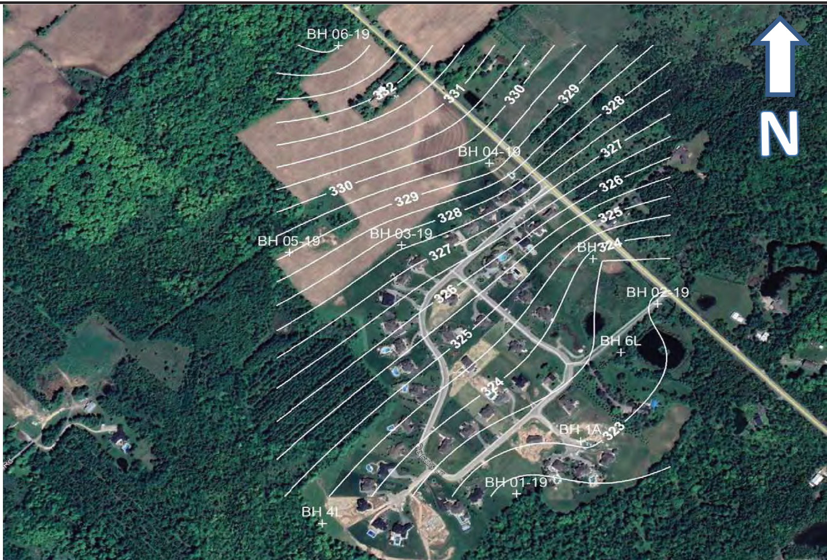
Drawing 3 - Groundwater Contours - September 2020 Audrey Meadows Subdivision - Puslinch
