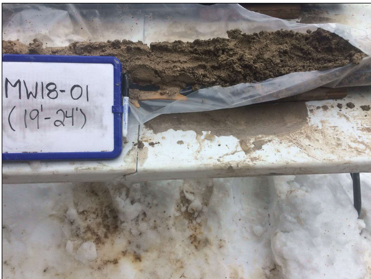
Core Photo: MW18-01 Depth: 19' - 24'
